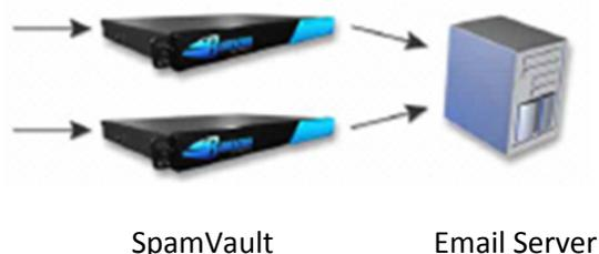
**Figure 2: Level 2 Redundancy Setup**
