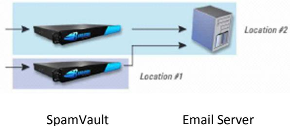
**Figure 4: Recommended Redundancy Setup**
